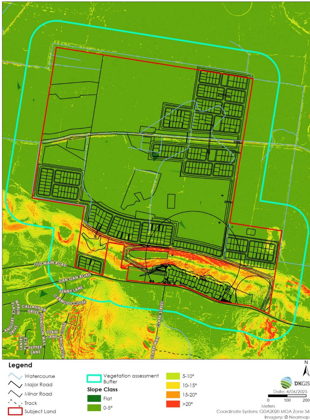
Figure 17: Slope Assessment at Development Footprint
