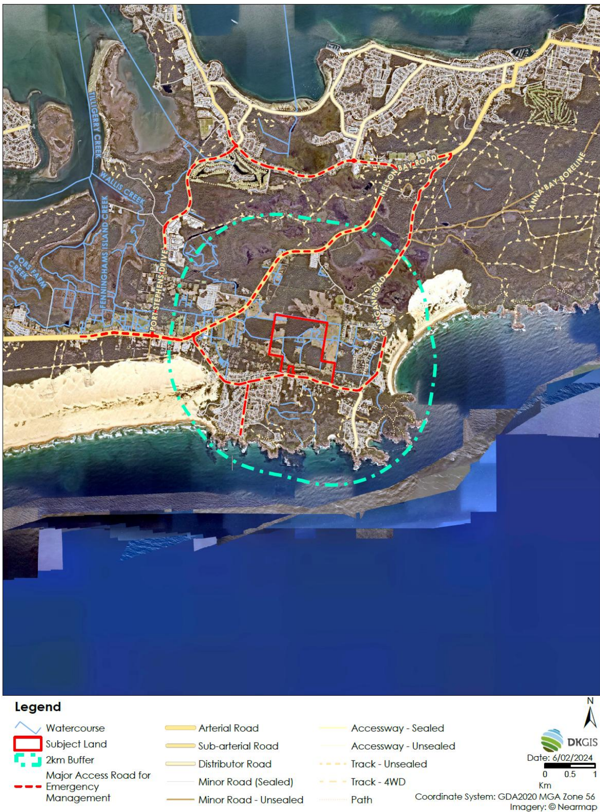
Figure 31: Existing Access and Egress
